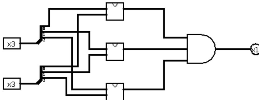
Figure 3: The complete equality circuit.
