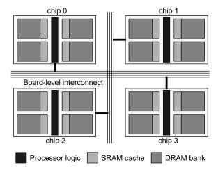
Figure 5. A unified processor/DRAM system
