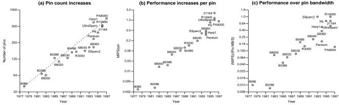
Figure 1. Physical microprocessor trends
