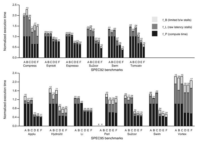
Figure 3. Effect of latency-reduction techniques
