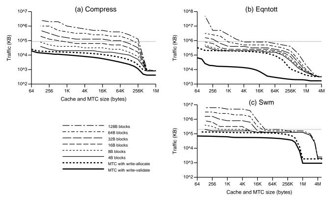
Figure 4. Total traffic generated by different cache and MTC sizes
