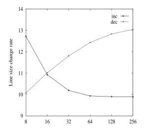
Figure 8: % misses producing line size change in GCC
