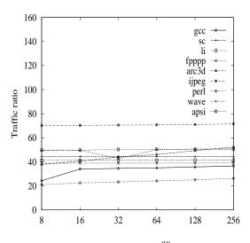
Figure 10: Fetch traffic ratio  $R_T^{32}$  to 32B fixed case
