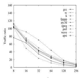
Figure 9: Fetch traffic ratio  $R_T^l$  to same-size fixed case
