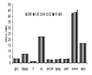
Figure 5: Miss rate vs initial adaptive line size
