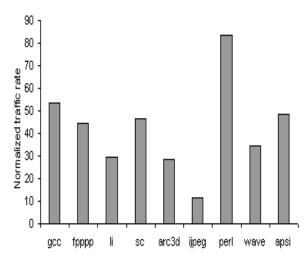
Figure 14: Traffic difference  $\Delta T_8^{16}$ : tag per 8B vs 16B
