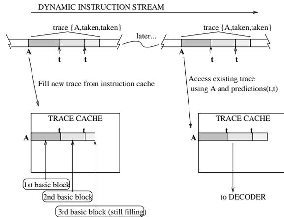
**Figure 2. High level view of the trace cache.**
