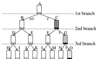
**Figure 6. BAC stores subgraphs of the CFG.**
