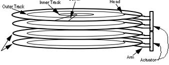
Disk Latency = Queuing Time + Controller time + Seek Time + Rotation Time + Xfer Time
