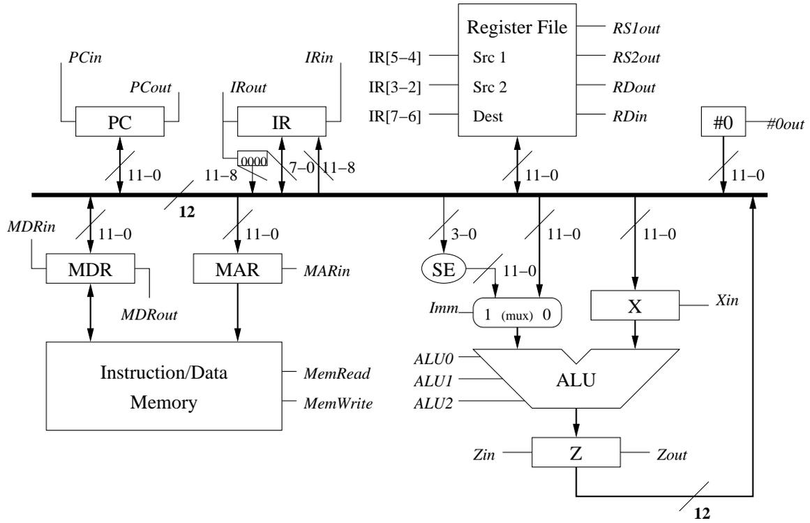
[9] Fill in the microcode steps necessary to perform an instruction fetch (incrementing the PC is considered part of the instruction fetch process).
