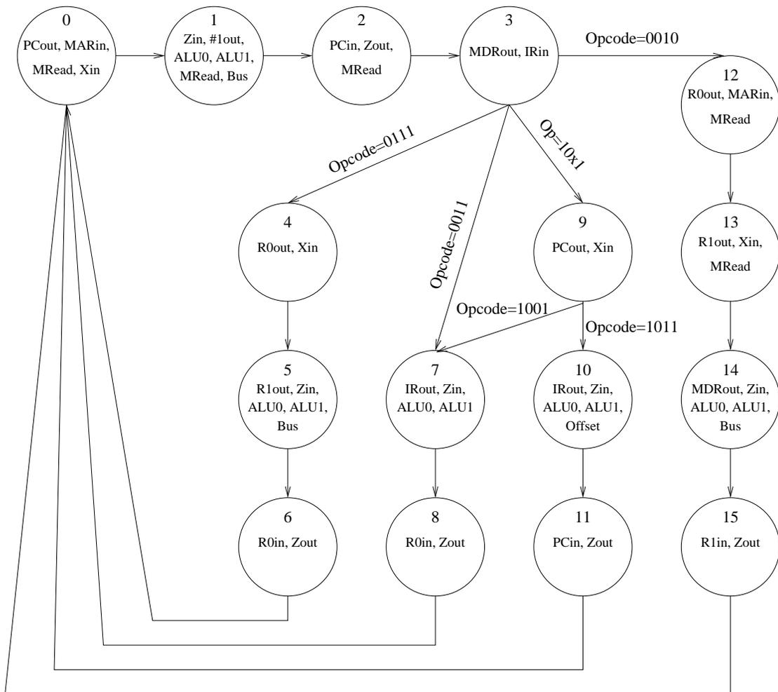
[3] Assuming there are 4 state variables ( $Y_3$ - $Y_0$ ), that  $\text{State0} = \overline{Y_3} * \overline{Y_2} * \overline{Y_1} * \overline{Y_0}$  (0000) and  $\text{State15} = Y_3 * Y_2 * Y_1 * Y_0$  (1111), write down the exact boolean equation for the **MDRout** signal.
