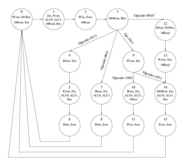
[4] Assuming there are 4 state variables (Y3-Y0), that State0 =  $\overline{Y3}*\overline{Y2}*\overline{Y1}*\overline{Y0}$  (0000) and State15 = Y3\*Y2\*Y1\*Y0 (1111), write down the exact boolean equation for the **Bus** signal.
