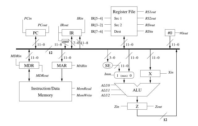
[6] Fill in the microcode steps necessary to perform an instruction fetch (incrementing the PC is considered part of fetch).
