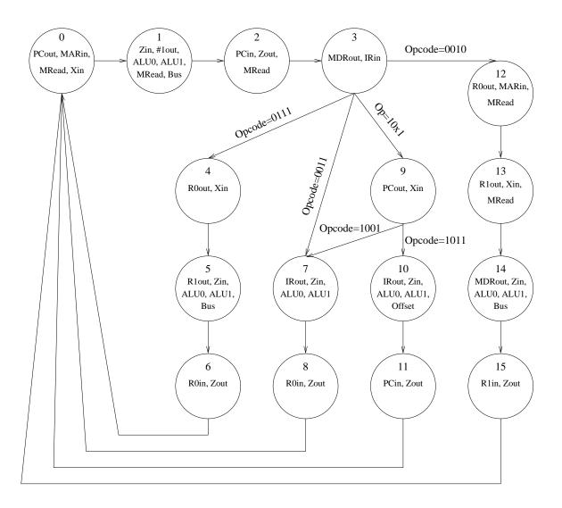
[3] Assuming there are 4 state variables (Y3-Y0), that State0 =  $\overline{Y}3*\overline{Y}2*\overline{Y}1*\overline{Y}0$  (0000) and State15 = Y3\*Y2\*Y1\*Y0 (1111), write down the exact boolean equation for the **R1out** signal.
