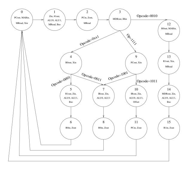
[4] Assuming there are 4 state variables (Y3-Y0), that State0=!Y3\*!Y2\*!Y1\*!Y0 (0000) and State15=Y3\*Y2\*Y1\*Y0 (1111), write down the exact boolean equation for the **PCout** signal.
