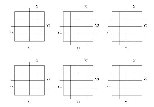
11. (15 pts) Given the following Karnaugh maps, implement the sequential machine using an SR FF for Y1, a JK FF for Y2, and a T FF for Y3. You do not need to draw the gates, but you do need to write down the **minimized** input equations for each of the inputs of each of the Flip Flops in the circuit.
