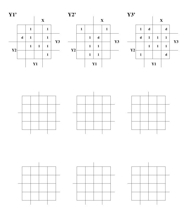
13. (10 pts) There's a machine, it's coin-operated, it does something, blah blah blah. Two kinds of coins, X1 (worth 2) and X2 (worth 1), can't put both in simultaneously. Machine requires sum of 3 in order to do its thing. The machine must give change.
