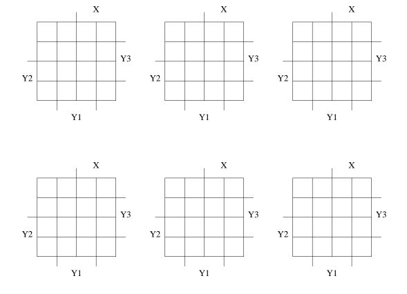
18. (15 pts) Given the following Karnaugh maps, implement the sequential machine using a JK FF for Y1, an SR FF for Y2, and a T FF for Y3. You do not need to draw the gates, but you do need to write down the **minimized** input equations for each of the inputs of each of the Flip Flops in the circuit.
