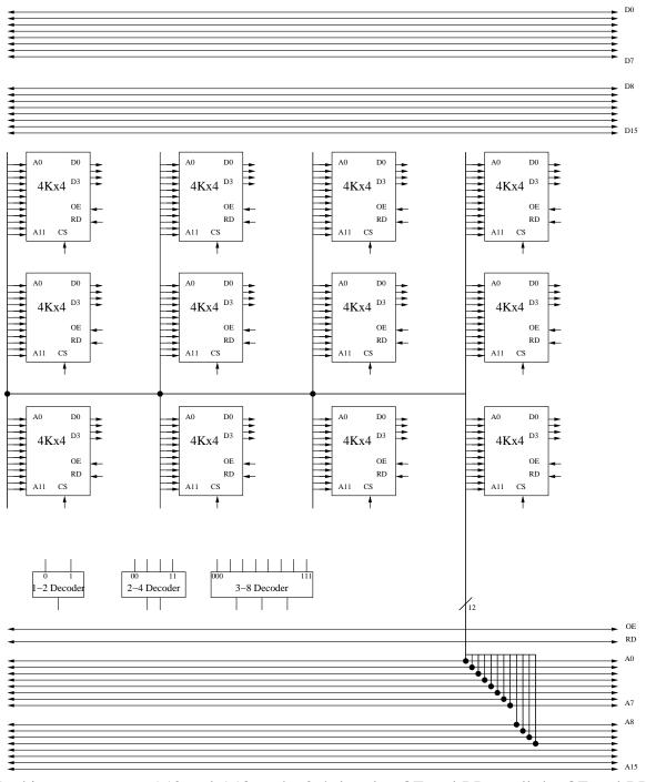
In this case, connect A12 and A13 to the 2-4 decoder, OE and RD to all the OE and RD lines on the chips, and then the 00 line from the decoder to the CS of 4 different 4Kx4 chips, the 01 line to another group of 4 CS lines, and the third output of the 2-4 decoder to the third group of 4 chips. Each group of 4Kx4 chips will provide 4Kx16 outputs if you connect their outputs to the data bus correctly.
